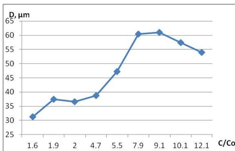
Fig. 4. Dependence of size of calcium sulphate particles on solution supersaturation degree at 1-step conversion
