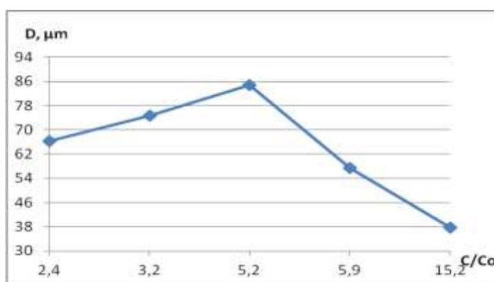
Fig. 5. Dependence of size of calcium sulphate particles on solution supersaturation degree at 2-step conversion
