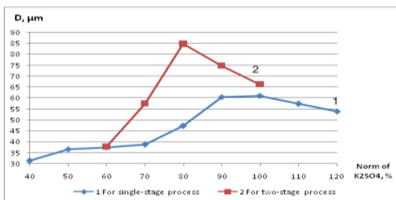
Fig. 3. Conversion mode influence on average diameter of calcium sulphate particles
