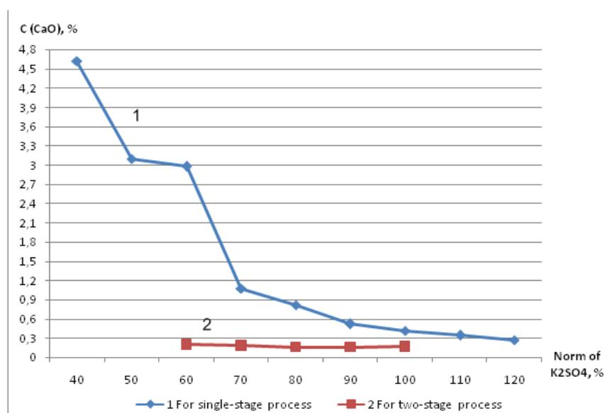
Fig. 1. Dependence of CaO content in a conversion solution on potassium sulphate solution norm
