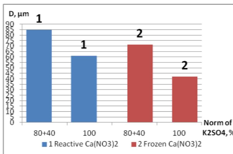
Fig. 7. Comparison of filtration productivity for suspension obtained from reactive (1) and frozen out calcium nitrate (2)
